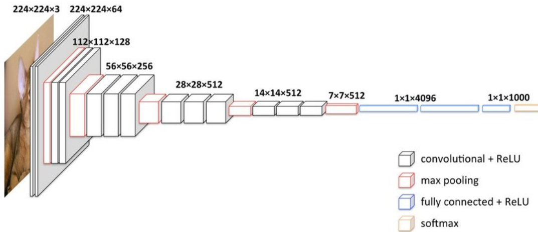
Figure 1: VGG-16 model architecture (Courtesy of Shi, et al., DOI:10.1117/12.2293594)
